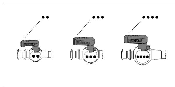
The stopcock housings and the corresponding stopcock inserts are marked with indicator nubs in order to simplify assembly.
